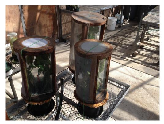
**Figure 5**. Wood frame cages covered with Dacron fabric and with a glass side. The wooded frames here have lasted 60 years.
